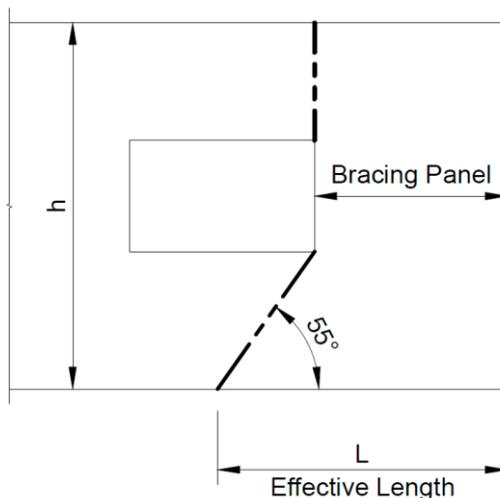
**Figure 7.3: Effective length of bracing panel with a single window**
