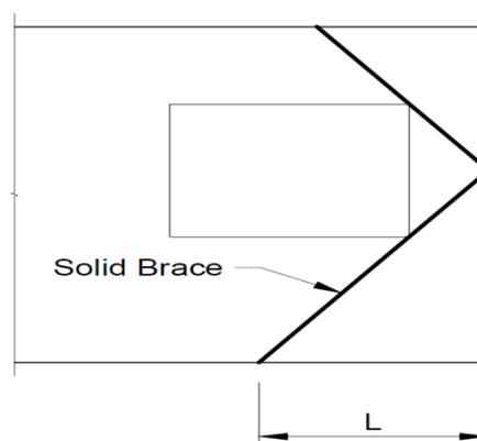
**Figure 7.2: Solid Bracing around Windows with Dog-leg Brace**
