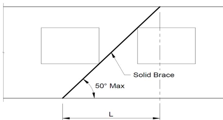
**Figure 7.1: Bracing around Windows**
