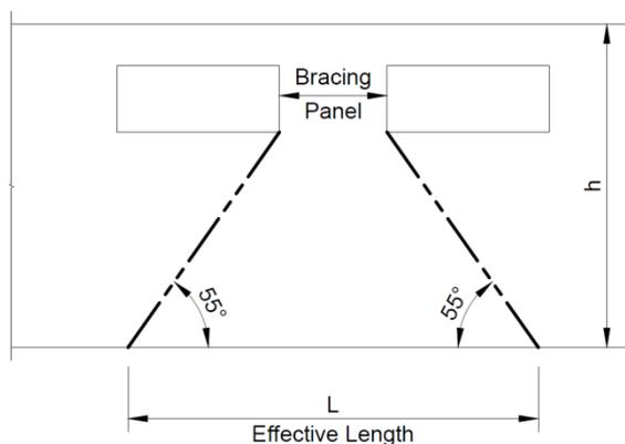
**Figure 7.4: Effective length of bracing panel with double windows**
