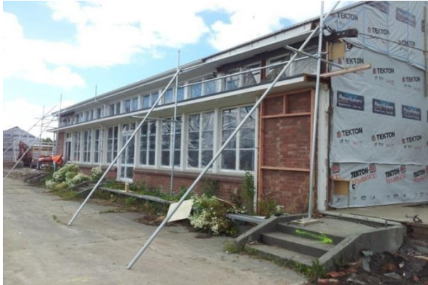
Figure 6. The Dominion block in early stages of the longitudinal test
