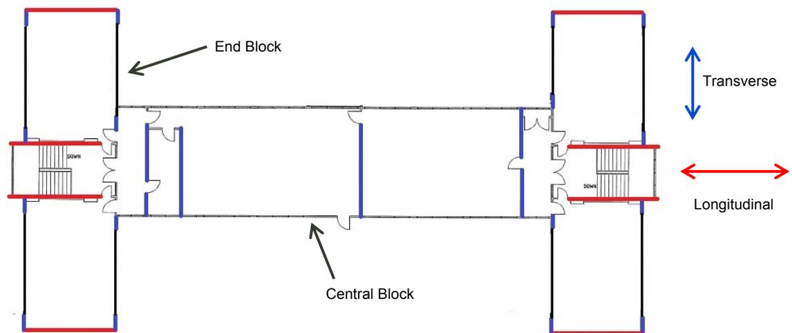
Figure 1 - Typical Nelson Block Bracing Layout - First Floor
