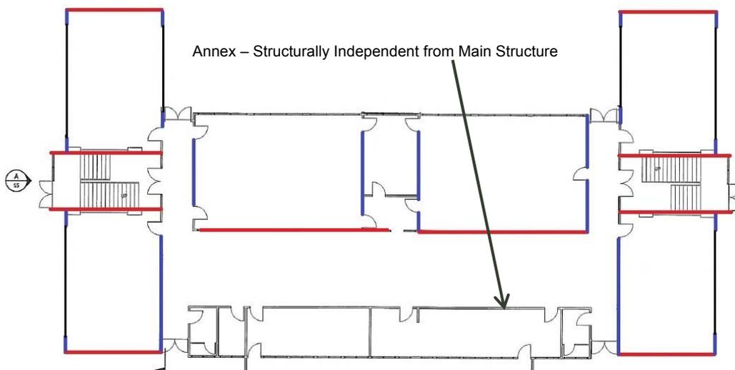
Figure 2 - Typical Nelson Block Bracing Layout - Ground Floor
