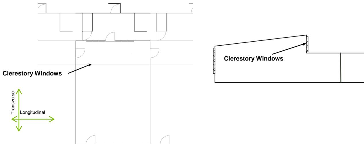
Figure 1 – Typical Avalon Block Plan View (left) and Side Elevation (right)
